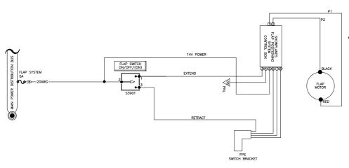
Note: For RV (4,6,7,9) connector motor P-1 to red wire and P-2 to black wire.
